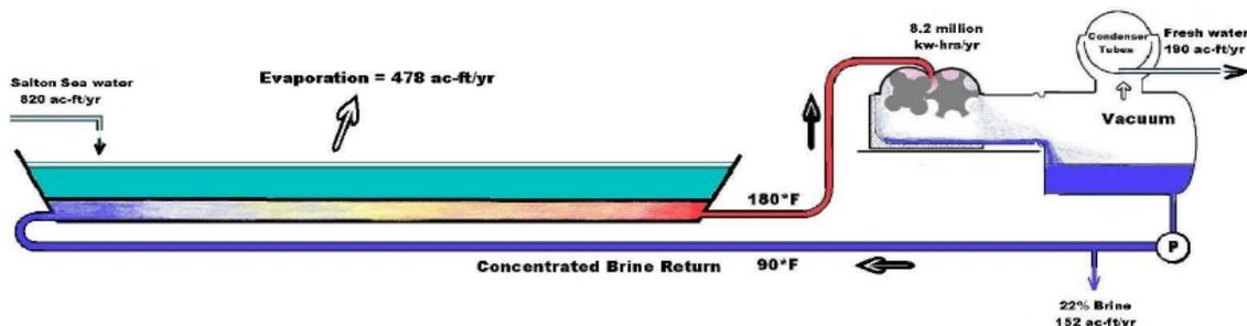
Hot bottom layer brine from the pond flows into the expander which drives a generator to produce electricity. Pond and expander and rates are sized so as to drive a 1-MW synchronous generator for electricity production. Steam exiting the expander is condensed, yielding distilled water, and the residual brine is more concentrated than was drawn from the pond.
